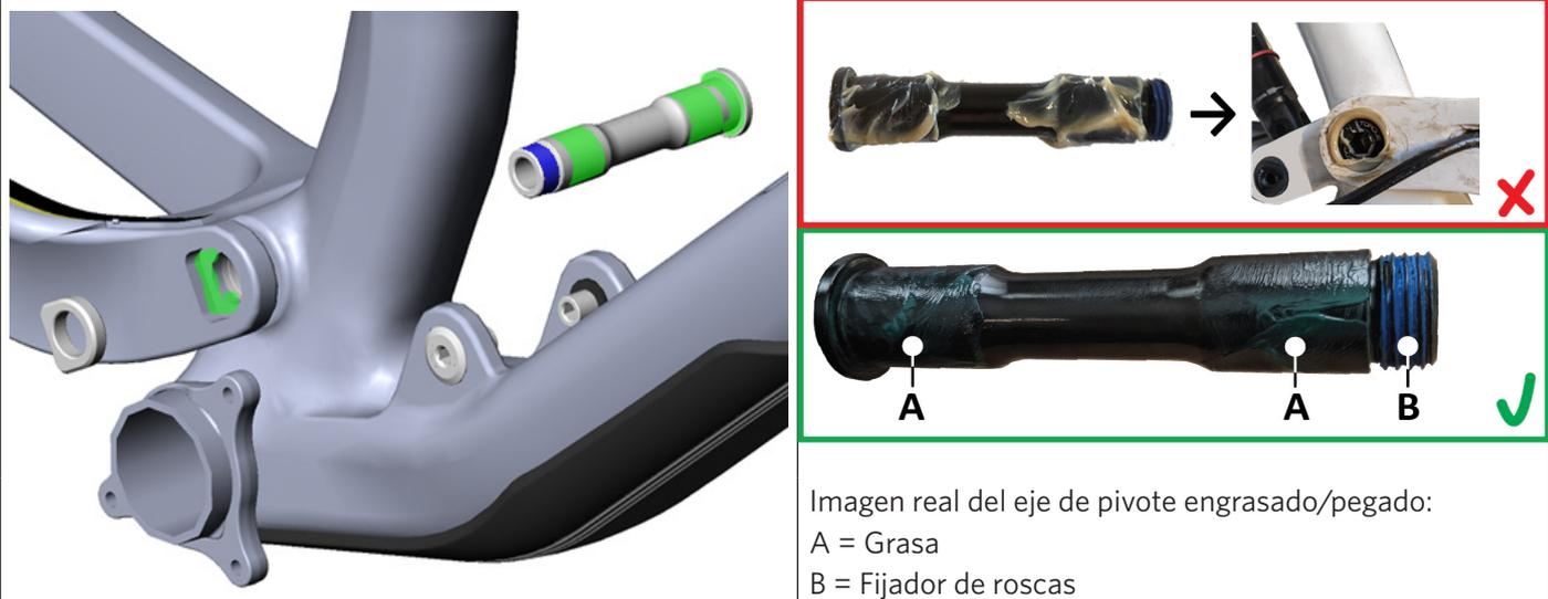
The diagram on the left shows a grey bicycle frame with a green and blue axle. To the right, a red-bordered box shows an incorrect application of grease, with a red 'X' mark. Below it, a green-bordered box shows the correct application of grease (A) and lock compound (B) on the axle, with a green checkmark. A legend below the green-bordered box reads: "Imagen real del eje de pivote engrasado/pegado: A = Grasa B = Fijador de roscas".
