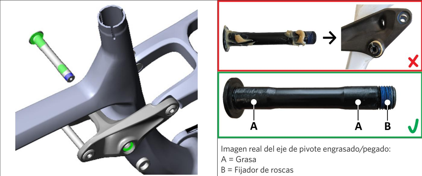
The diagram on the left shows a grey bicycle frame with a green and blue axle. To the right, a red-bordered box shows an incorrect application of grease, with a red 'X' mark. Below it, a green-bordered box shows the correct application of grease (A) and lock compound (B) on the axle, with a green checkmark. A legend below the green-bordered box reads: "Imagen real del eje de pivote engrasado/pegado: A = Grasa B = Fijador de roscas".
